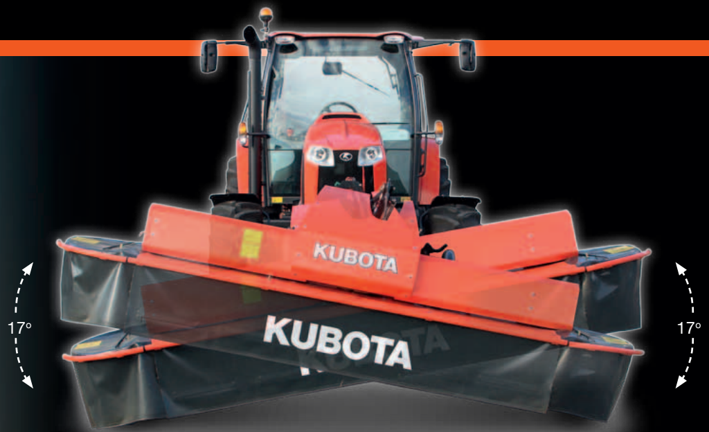
The mowing unit moves independently from the front linkage, ensuring the best possible pattern of movement and the transverse adaptation sets the standard in this segment.
