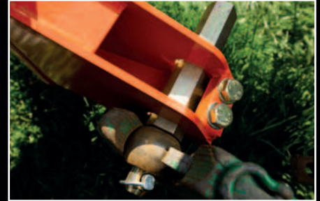
The linkage pins are easily adjusted to match the tractor width, which enables the mower to cut to its full working width.
