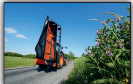
For transport the machine is folded hydraulically from the tractor cab to the vertical transport position well behind the tractor, ensuring a stable and steady transport.
