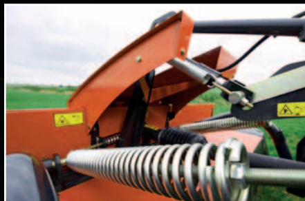
Two springs provide excellent ground following ability.
