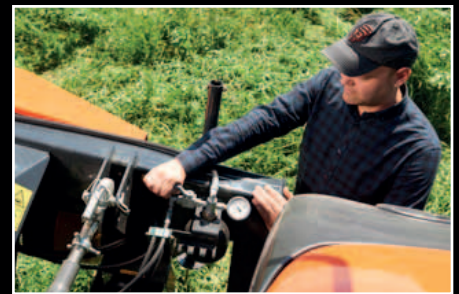
Hydraulic setting of ground pressure.
