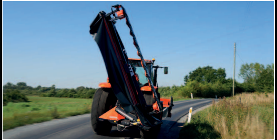
Up to 125° vertical transport position for excellent weight distribution.
