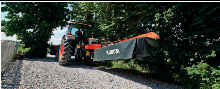
For transport the mower is swung hydraulically into horizontal position behind the tractor. Fast and easy conversion, with no need to leave the tractor.
