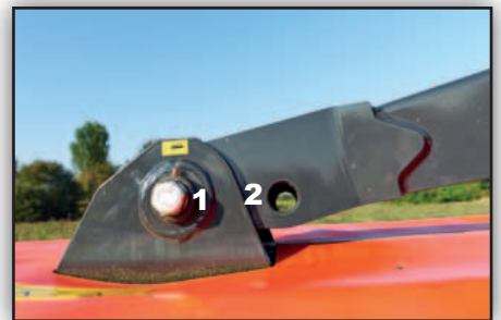
Two mounting options for optimal overlap with a front mounted machine.
