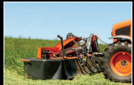
A BreakAway solution, integrated in the headstock, helps clear obstacles.
