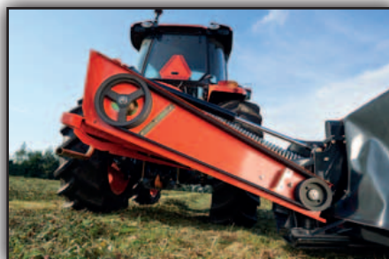
Four v-belts ensure excellent transfer of power.
