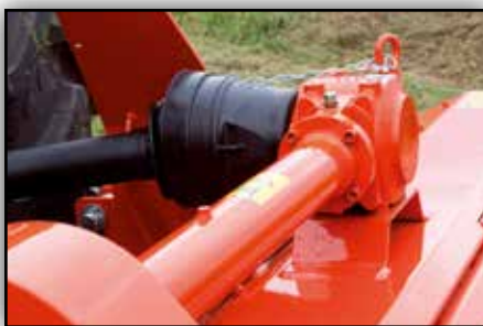
Gearbox with integrated free wheel
