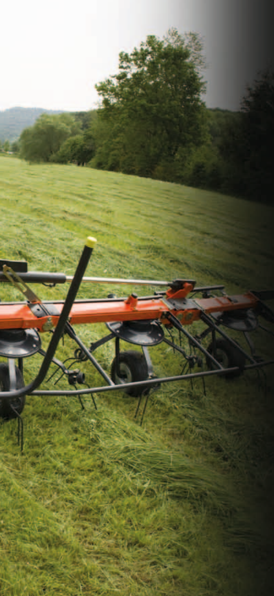
Large 18.5" wheels under centre unit to compensate for additional weight of carrier, improving running characteristics and leading to less soil contamination.
