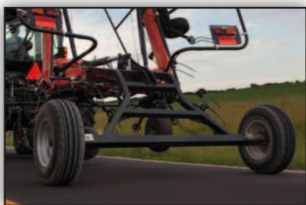
A wide track on the transport carrier ensures excellent running characteristics.
