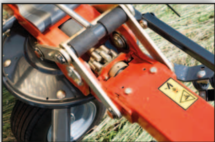
HexaLink finger clutch permits the rotors to fold 180° for transport.
