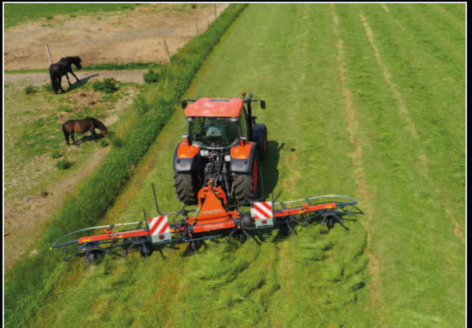
Keep the crop inside the field with border tending, tending the crop away from the border line.
