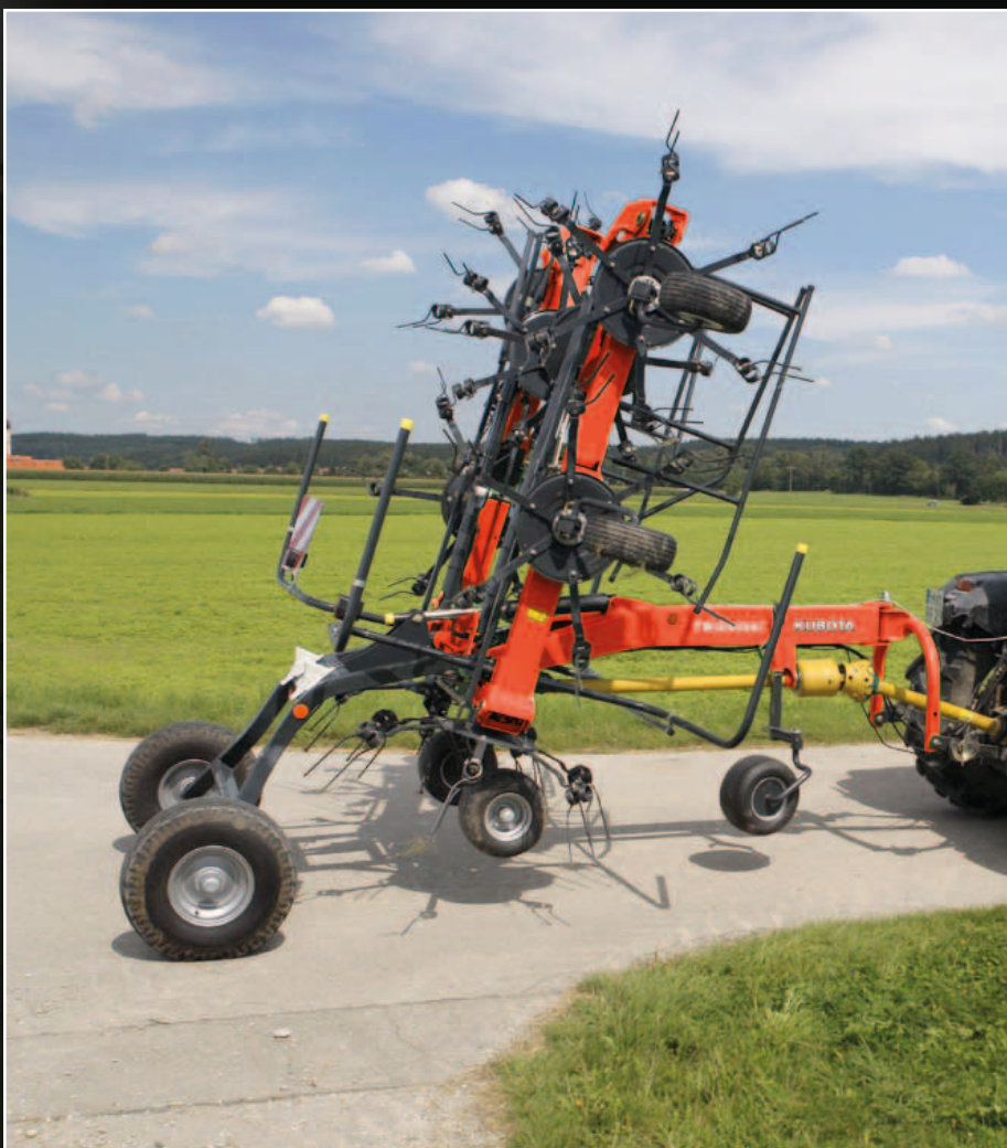
Large 18.5" wheels under centre unit to compensate for additional weight of carrier, improving running characteristics and leading to less soil contamination.
