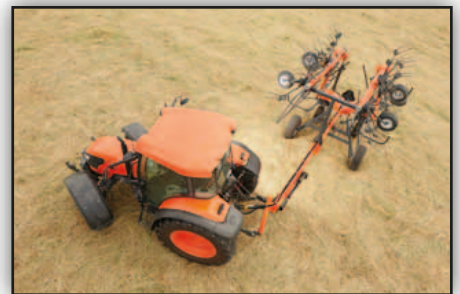
80° turning angle ensures excellent manoeuvrability.
