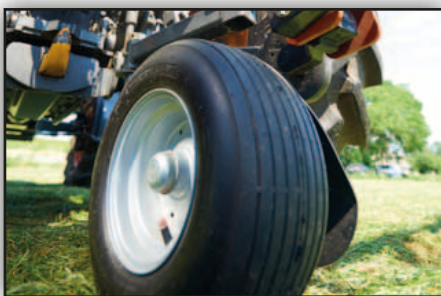
All tedders can be equipped with a third wheel to ensure correct set up of the tedder interdependent from tractor and driver.
