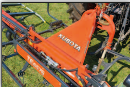
Strong and sturdy mainframe design with V-shaped central unit.
