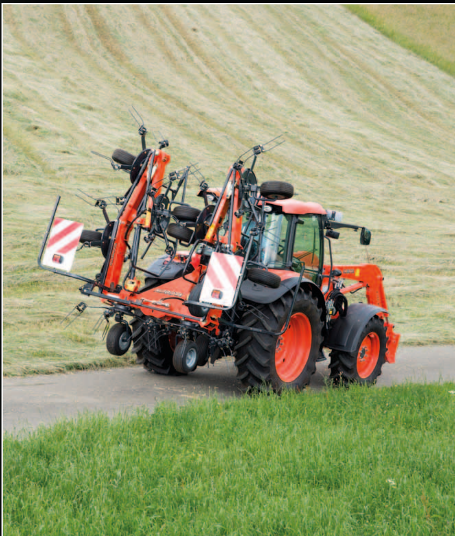
TE8080 folds into a very compact position for transport.
