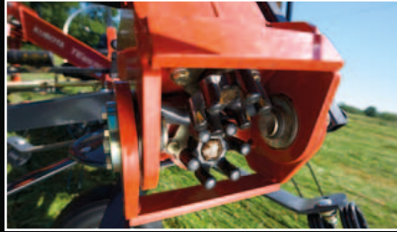
Kubota HexaLink finger clutch permits a 180° folding of the rotors for transport.
