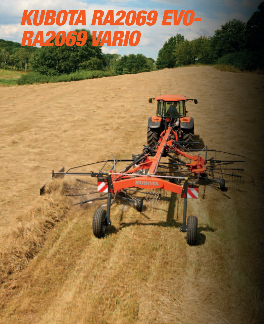
Generous overlap between rotors ensures clean raking.
