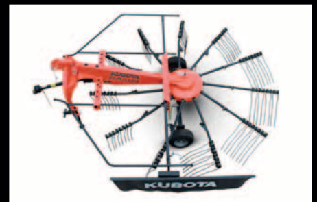
RA1039 – 3.90m working width, weighing 460kg.
