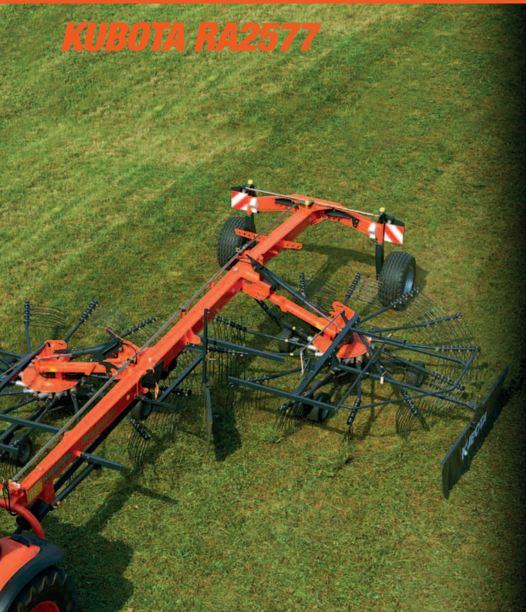
The low position of the rear frame, with low gravity point, ensures excellent stability.
