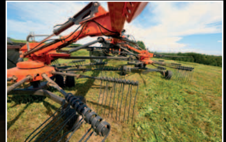
Generous overlap between rotors ensures clean raking.
