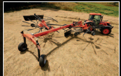
RA2069 features a headstock that turns through a 80° angle for superior manoeuvrability.
