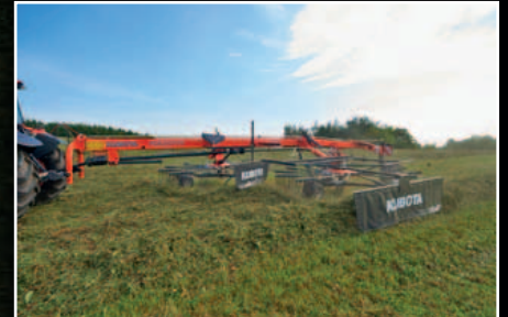
The low position of the rear frame, with low gravity point, ensures excellent stability.
