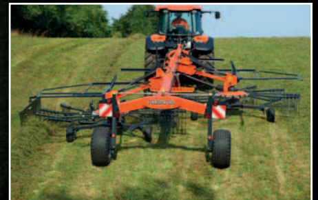
The side delivery concept allows you to collect crop from 15.00m into a single swath.
