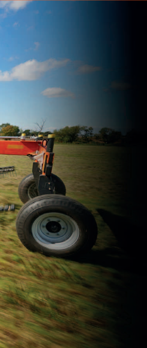
With 9.00m working width and transport height below 4.00m, even without detaching tine arms...
