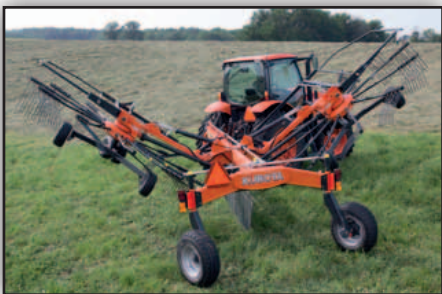
The ability to make sharp turns up to 80° and the cross stabilizer in the headstock are Kubota features.
