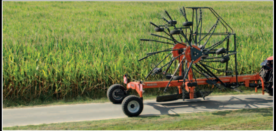
With 9.00m working width and transport height below 4.00m, even without detaching tine arms...
