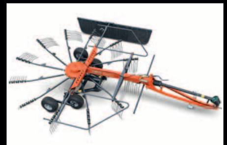
RA1047T – 4.70m working width and a weight of only 665kg.
