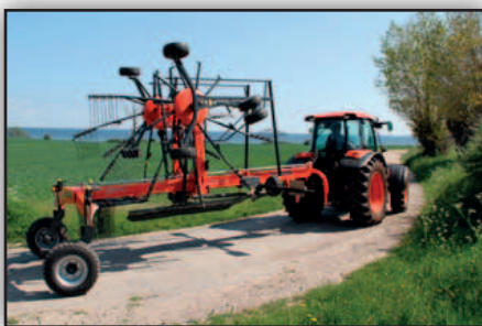
To limit transport height further the tine arms can be removed on RA2076. The swath board folds up automatically.
