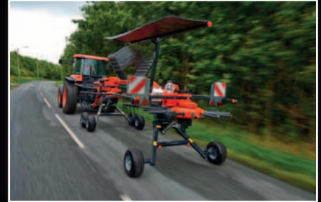
Pulled axles for smooth running characteristics and reduced power requirement.
