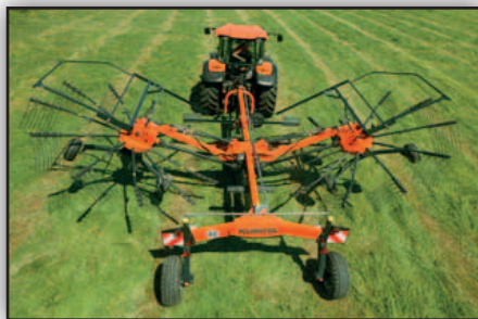
The hydraulic adjustable rotors on RA2076 can be set between 7.00m...
