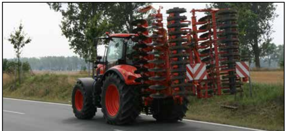
CD1500F: Transport width always below 2.50m ensure a safe road transport.
